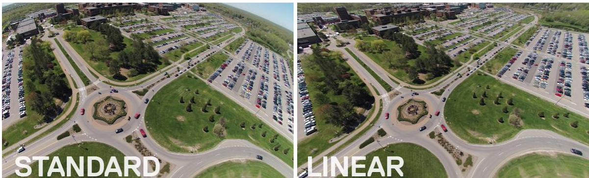
Figure 31. Comparison of Barrel Distortion Effects. Source: GoPro. (n.d.).
