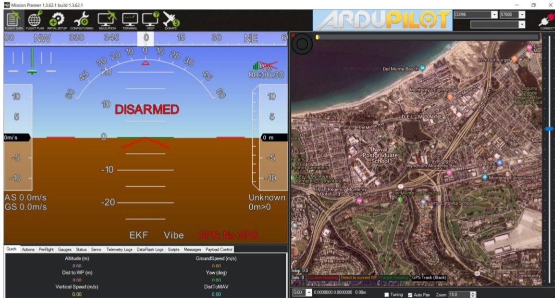
Figure 59. Screenshot of Telemetry Visualization in Mission Planner Software.
