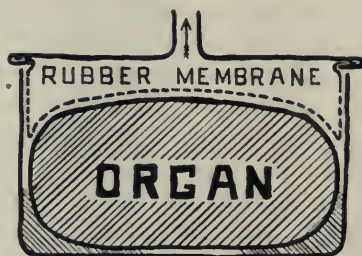
Fig. 1. Diagram showing construction of plate plethysmograph.
