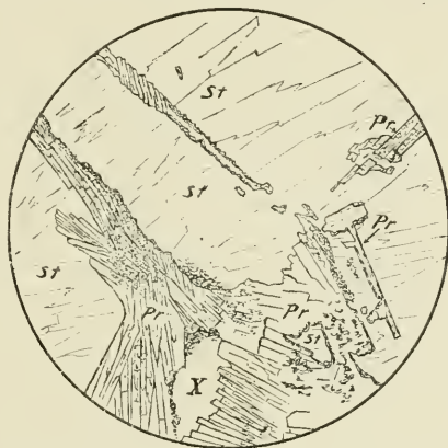
FIG. 21. Remnants of prehnite groups (Pr) in stilbite (St). \times 35 . Slide 74.
