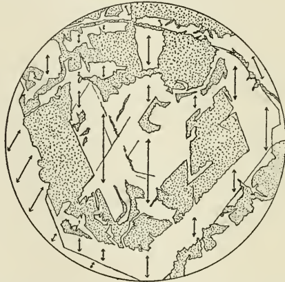
FIG. 12. Replacement of quartz (clear) by heulandite (stippled). Arrows show direction of vertical axes of quartz crystals. Many of the crystallographic lines approach parallelism, but few are strictly parallel. \times 35 . Slide 77.
