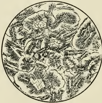
FIG. 1. Microlitic growth of phenocrysts in vitrophyric crusts. \times 35 . Slide 132.
