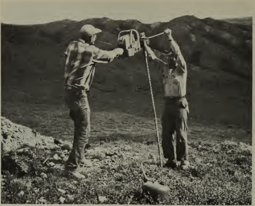
A small gasoline motor powers a drill used by Bureau of Mines to penetrate permafrost in Alaska's Kuskokwim River area in quest of mercury ore.
