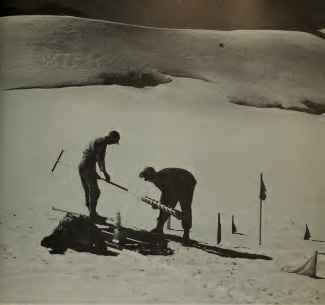
Glaciologists taking snow cores from a Glacier in western United States to obtain profiles of snow density, hardness, grain size, wetness, and dirt content.
