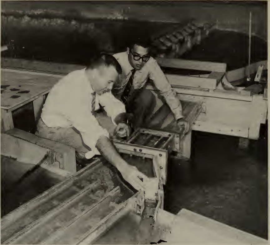
Engineers operate sluice gate of model in Bureau of Reclamation research laboratories in Denver.
