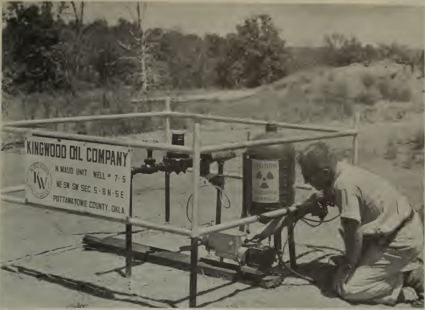
Water containing radioactive hydrogen is fed by a Bureau of Mines engineer into an Oklahoma oil well as part of a study on secondary recovery of petroleum.
