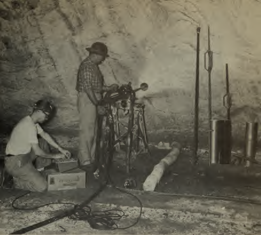
A device for measuring the stress in walls and pillars of underground mines is used by Bureau researchers at a commercial operation.
