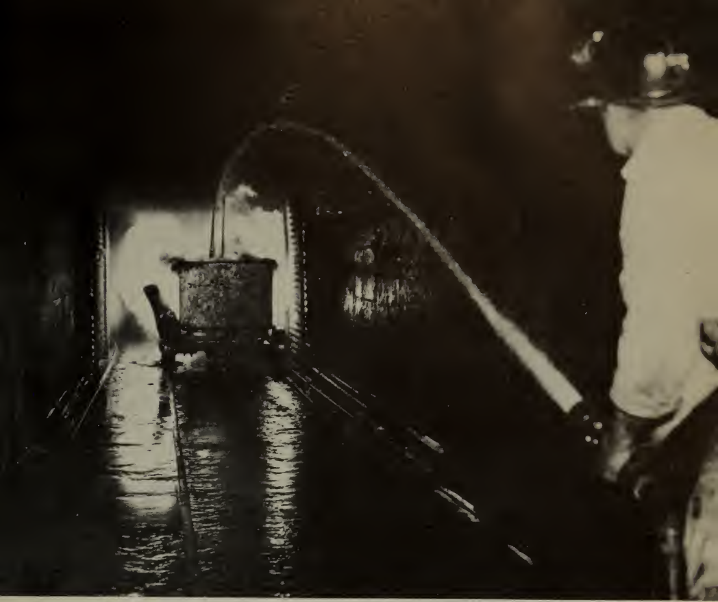
Purposely set fire in Bureau's experimental mine is fought with water during research on reducing hazards in coal mining.
