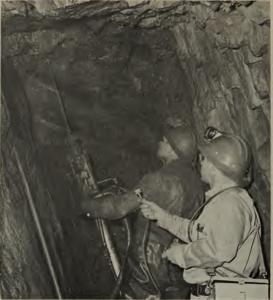
Radiation hazards in uranium mines were studied by the Bureau of Mines in cooperation with the Public Health Service. A Bureau engineer (right) collects radon-daughter products from the atmosphere.
