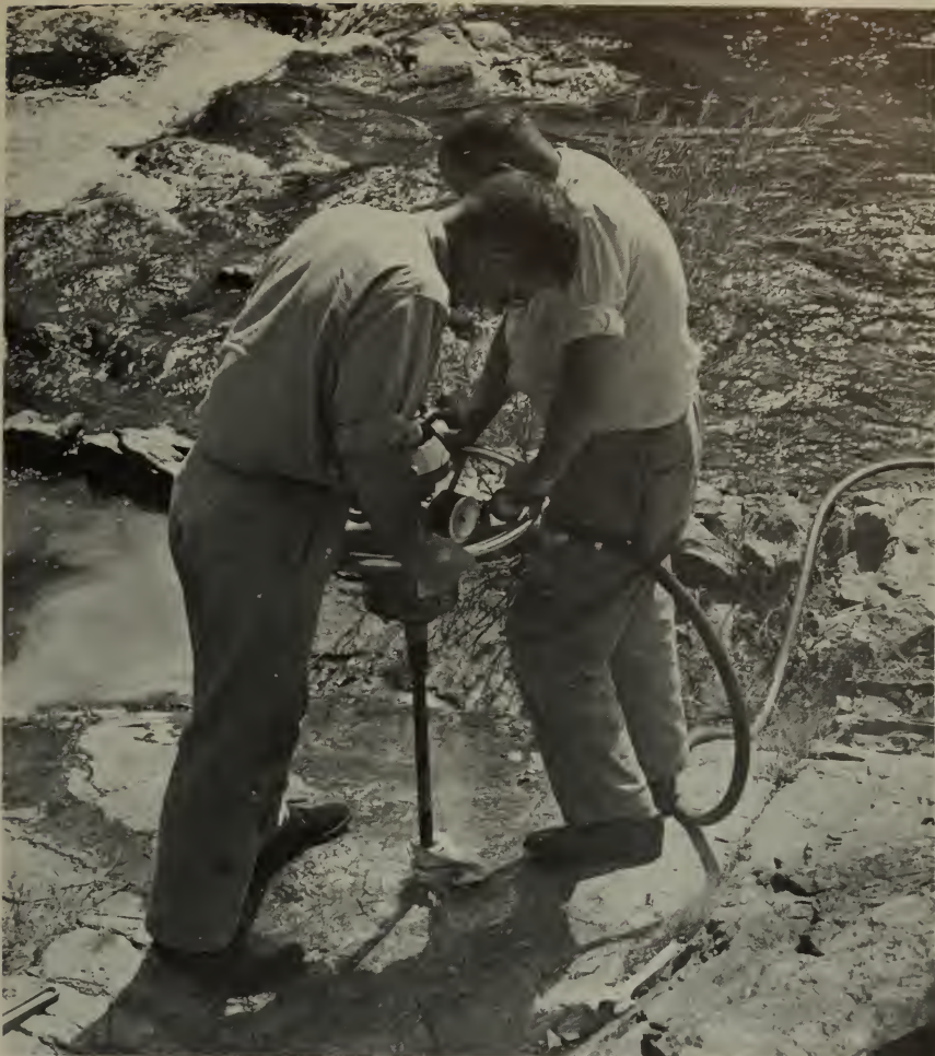
Geologists of the Survey use small portable core drills in collecting unweathered rock samples for geochemical analysis.
