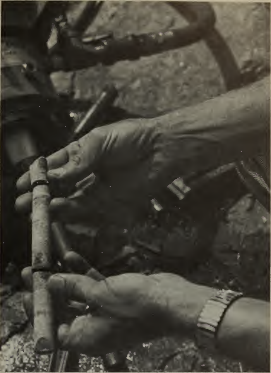
Survey geologists use small portable core drills to reach below the surface and gather unweathered rock samples for geochemical analysis.
