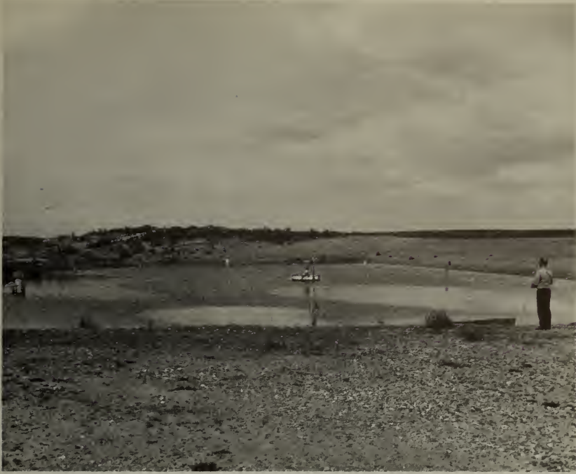
Interior Department hydrologist watching the spread of a thin film of octadecanol (a floating waxy fluid for the suppression of evaporation in small reservoirs). The scene is a small stock tank near Laredo, Tex.
