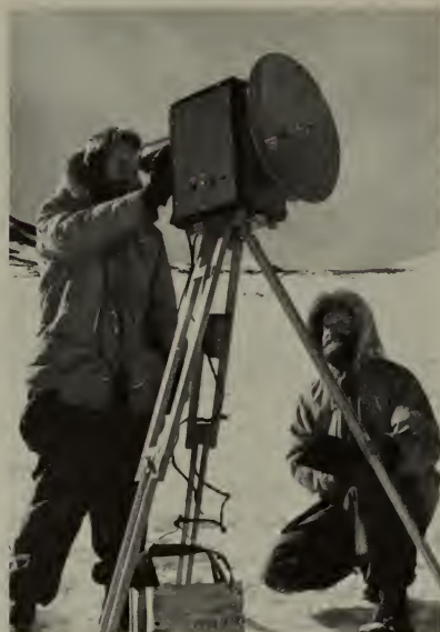
Topographic engineers of the Geological Survey use the latest electronic distance measuring devices in mapping Antarctica.
