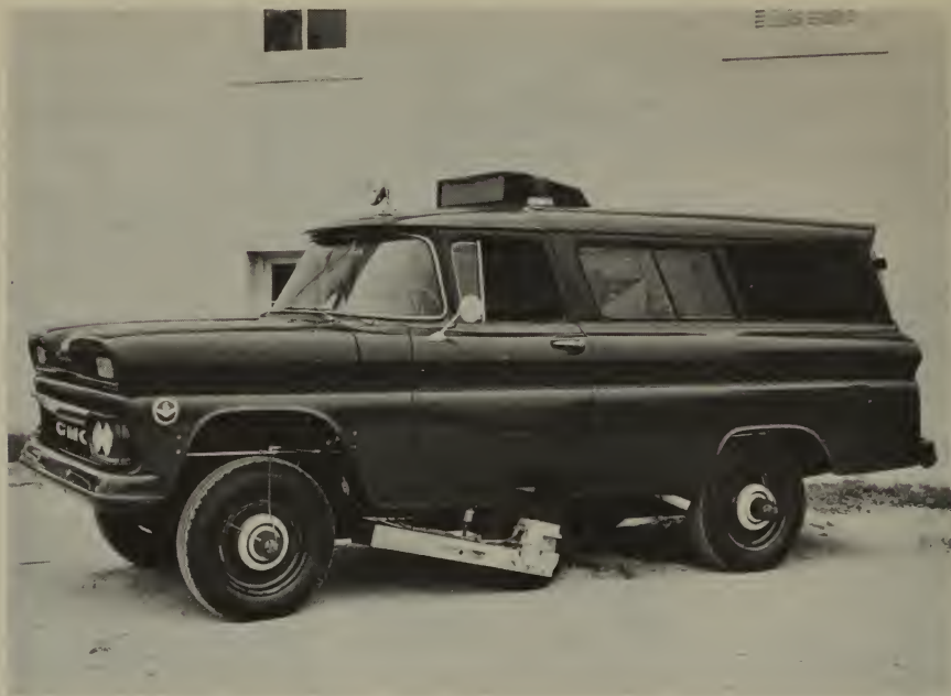
The Geological Survey's new self-propelled electronic elevation meter automatically measures ground elevations. It is virtually a computer on wheels.
