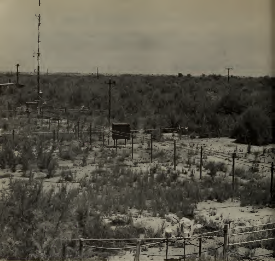
Saltcedar study site near Buckeye, Ariz., before the reestablishment of vegetation. The tall mast carries instruments to measure wind, temperature and humidity profiles. The shorter mast supports radiation measuring devices.
