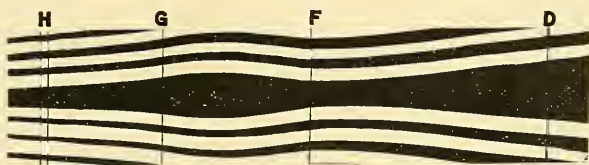
FIG. 5. Interference dispersion curves from a thin film of concentrated alcohol-fuchsine solution. Satisfactory cuts could not be made from original photographs.
