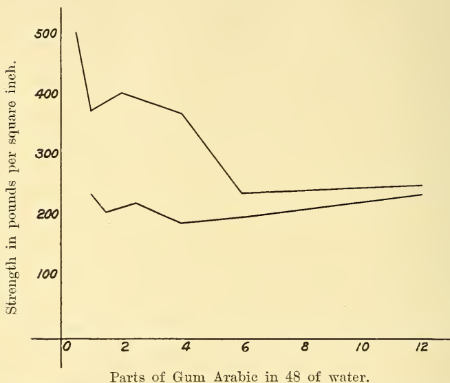
FIG. 3. Curves showing the effect of gum arabic solutions mixed with plaster of paris, based on test of 42 briquets.
