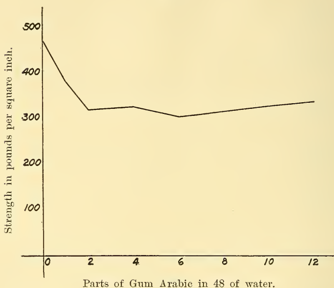
FIG. 5. The average of the curves of fig. 4, which is based on experiments with 108 briquets, soaked in solutions of gum arabic.
