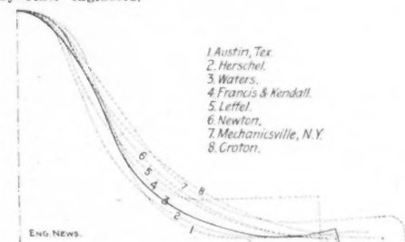
Cross-Sections of Eight Ogee-Faced Dams.
