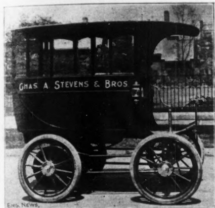
Fig. 3.—Electric Delivery Wagon in Use in Chicago, Ill. American Electric Vehicle Co., Chicago, Ill.
