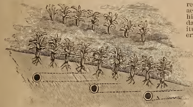
IRRIGATION ON SLOPE.—TILE LINES ALL ON DEAD LEVEL.
