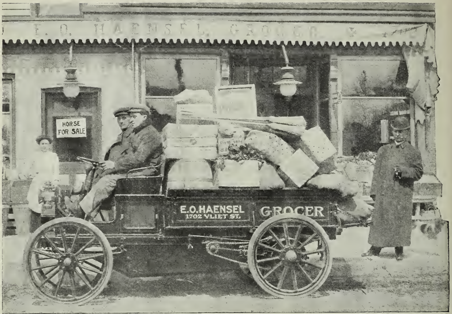
The Reo 1500-lb. truck which is equipped with a single-cylinder 12 h. p. motor, planetary transmission, and a 44x72 inch body.
