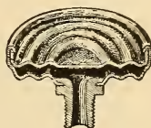
FIG. 22. Utica Capsular Spring.
