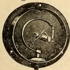
FIG. 16. Ashcroft Single Bourdon-Spring Steam Gauge.
