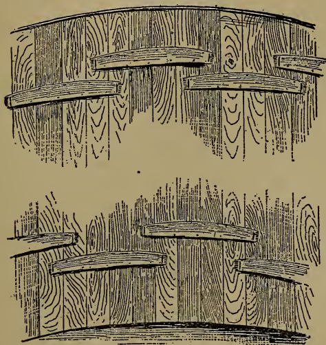
Fig. 18. Shows how barrel staves may be used in setting up a silo. They should be removed before the silo is filled.
