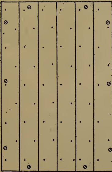
Fig. 7. Showing the construction of the door for the all-wood silo.
