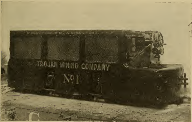
FIG. 56. Gasoline mine locomotive.
