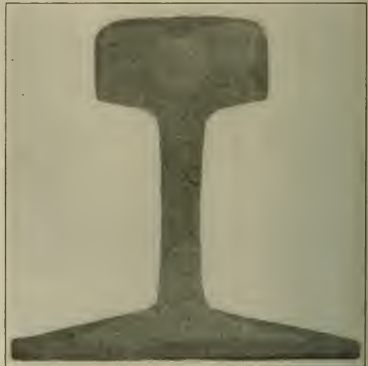
Fig. 3—Experimentally Formed Transverse Fissure. Located Centrally Over Web by Reason of Vertical Loading
