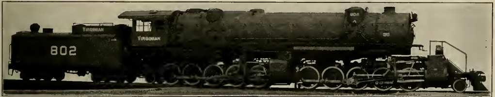
The Type of Mallet Locomotive, Weighing Approximately 450 Tons, Now in Service on the Virginian
