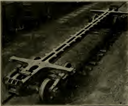
One-Piece Cast Steel Underframe Southern Pacific Box Car
