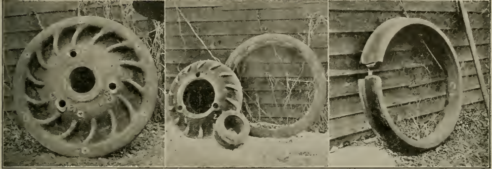
Cast Iron Wheel Showing Markings For Strain Measurements
