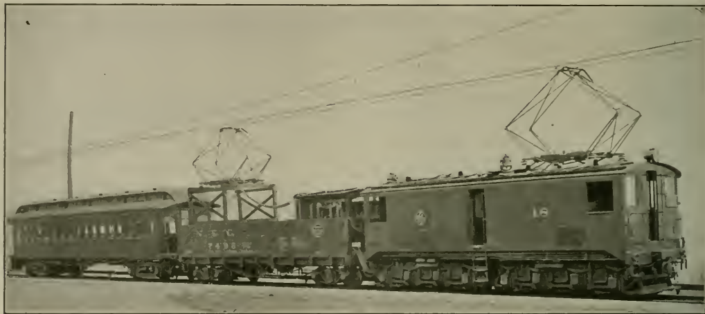
Train With Gondola and Observation Car Used in General Electric Company's Current Collection Tests
