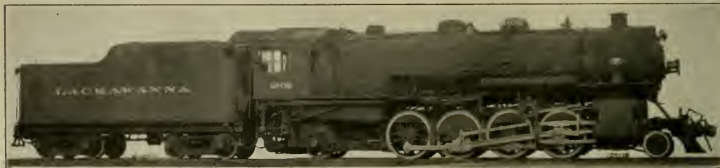
Mikado or 2-8-2 Type Locomotive on the Delaware, Lackawanna & Western. Built by American Locomotive Co.
