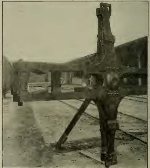
Bottom of One-Piece Cast Steel Underframe Showing Bolster and Center Plate
