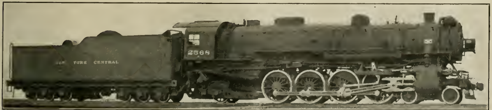
Three-Cylinder Mikado Type Locomotive of the New York Central—Built by American Locomotive Company
