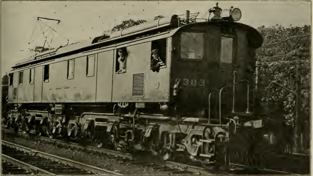
180-Ton Baldwin-Westinghouse Electric Locomotive, Now in Operation on the New York, New Haven & Hartford Railroad
