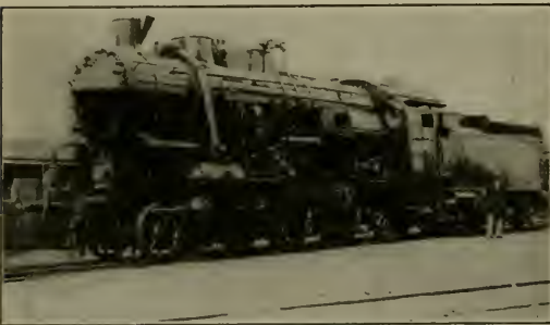
4-60 TYPE EXPRESS, LOCOMOTIVE FOR HUNGARIAN STATE RAILWAYS BUILT AT THE STATE RAILWAY SHOPS
