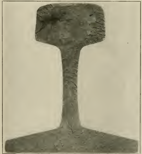
Fig. 2—Transverse Fissure in an Advanced Stage of Development
