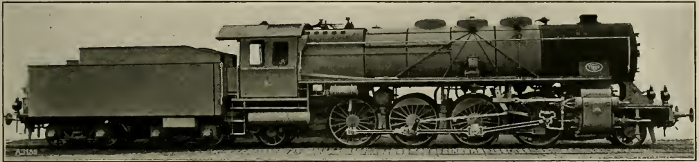
Mikado or 2-8-2 Type Three-Cylinder Locomotive of the German State Railways, Equipped With Superheater, Feed Water Pre-Heater and Purifier
