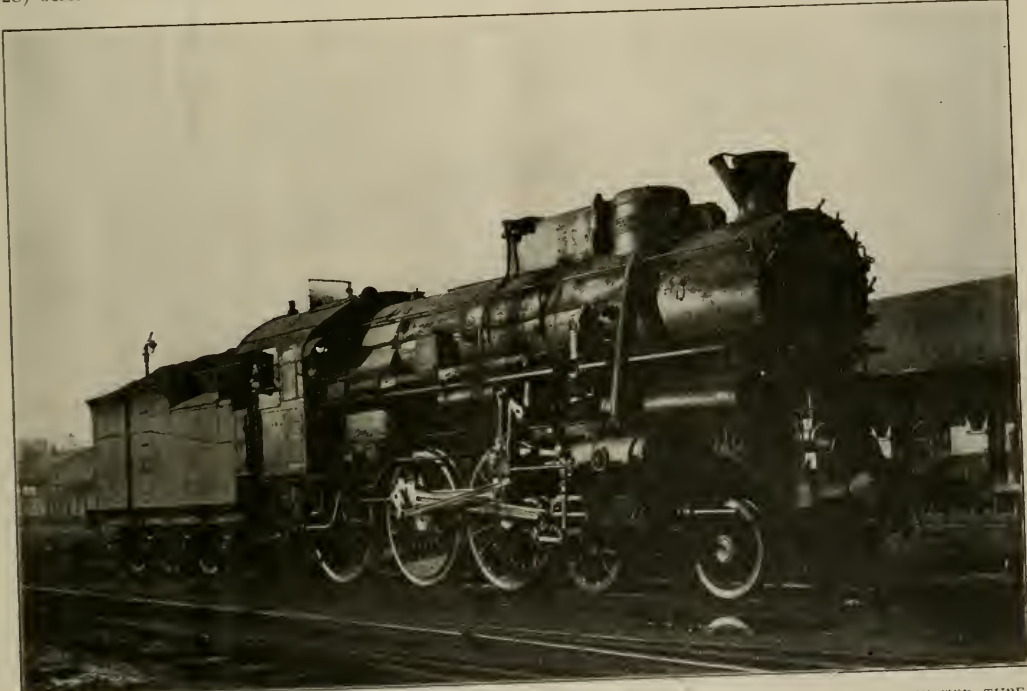
ROYAL HUNGARIAN STATE RAILWAYS 4-6-0 TYPE EXPRESS LOCOMOTIVE EQUIPPED WITH BROTTAN BOILER, WATER TUBE FIREBOX, LOOP WATER PURIFIER AND PREHEATER
