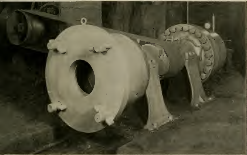
MACHINE FOR CASTING STEEL UNDER PRESSURE BY THE CENTRIFUGAL PROCESS IN A VERTICAL PLANE
