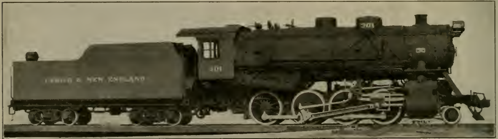
HEAVY CONSOLIDATION TYPE LOCOMOTIVE FOR THE LEHIGH & NEW ENGLAND RAILROAD. (Built by American Locomotive Co.)
