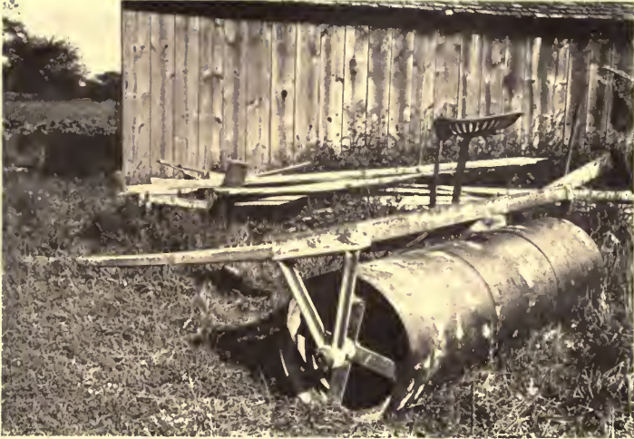
65. A THREE-SECTION IRON ROLLER
