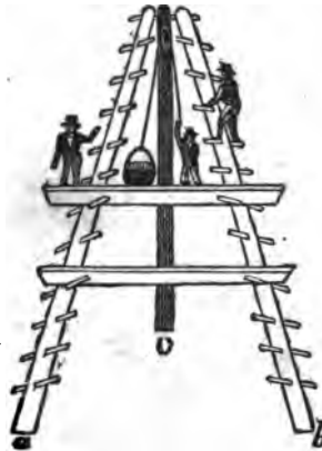
FIG. 153. French self-supporting orchard ladder.
