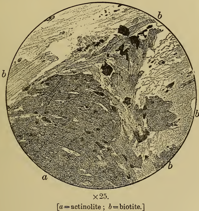
Fig. 6.—One end of a lancet-shaped crystal of actinolite, tipped and fringed with flakes of biotite. (From the ascent to the St. Gothard Pass.)
