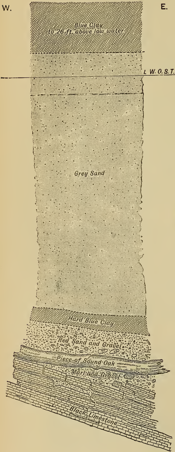
Fig. 4.—Section in cylinder at B.
