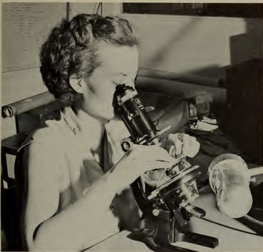
A Department geologist examining thin sections of potash ore with a petrographic microscope.
