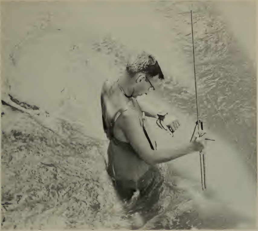
Survey geologist conducts velocity measurements as one step in determining the water discharge of a stream.
