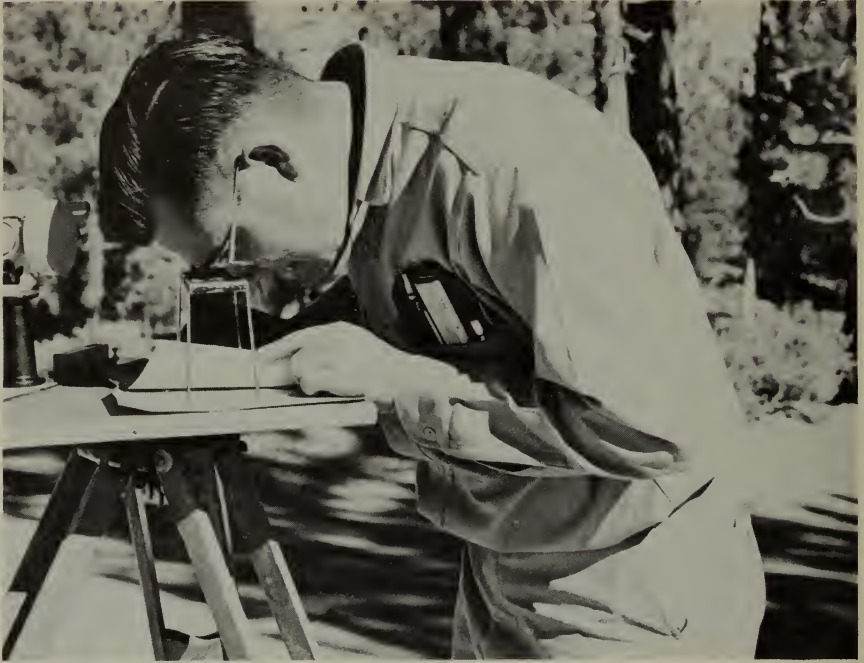
Aerial photographs are used here to establish elevations south of Lee Vining, California.
