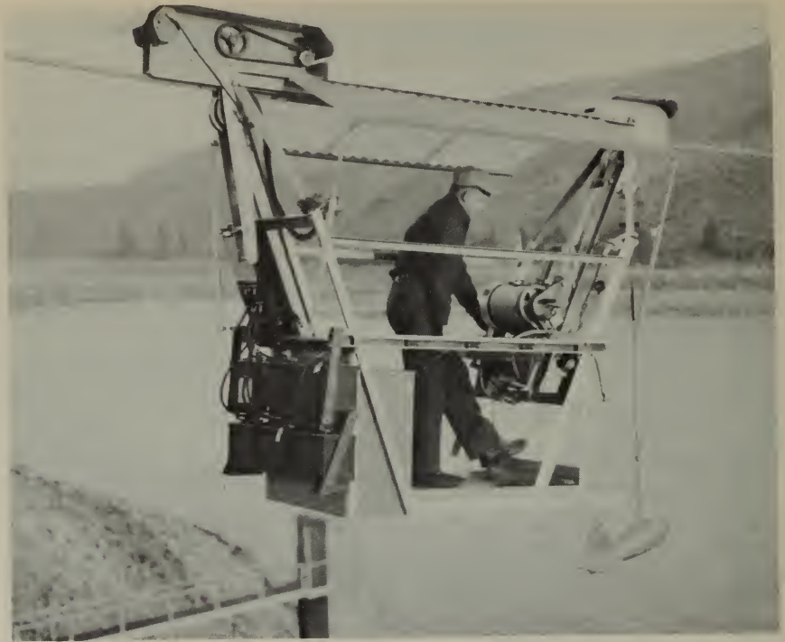
Geological Survey hydraulic engineer using a battery-powered cable car and sounding equipment to make streamflow measurements from a steel cable high above the Columbia River.
