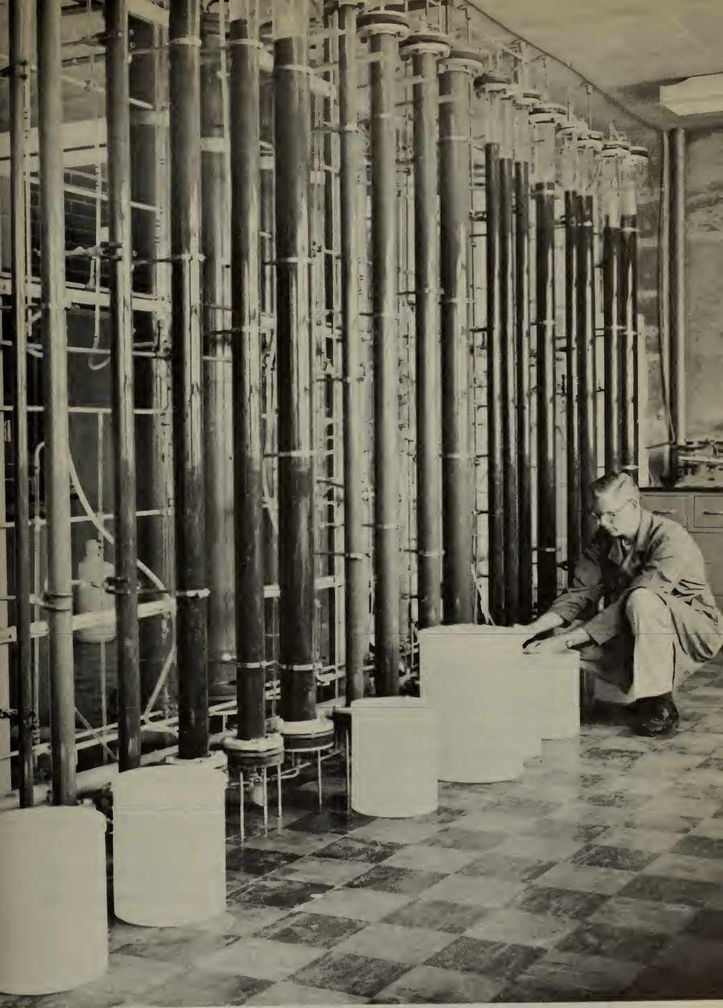
Operating ion-exchange columns, which are used in one of many approaches Bureau of Mines metallurgists are making to the problems encountered in separating closely associated metals.
