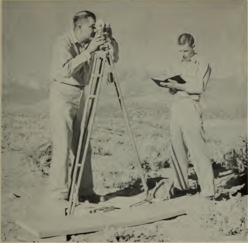
In a desert area east of the High Sierras in eastern California, engineers conduct control surveys for topographic mapping.
