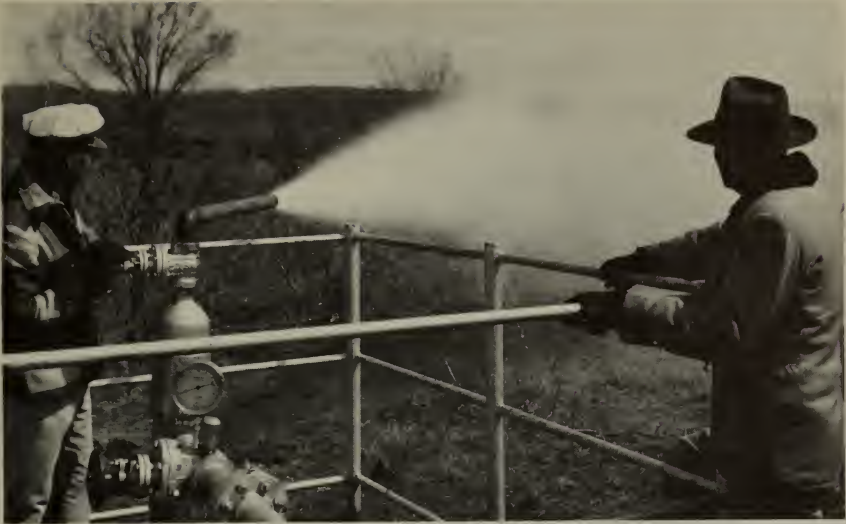
A jet of foam sprays from a wellhead during field tests of a technique devised by Bureau of Mines petroleum engineers for removing water from natural-gas wells with a column of detergent-generated foam.
