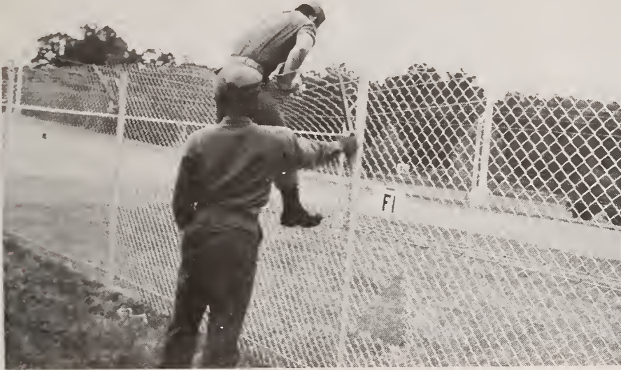
Figure 169. Outriggers, Still Attached to Barbed Wire, Cut, Pulled Down and Used as Hand and Foothold to Climb Over Fence; Test F1
