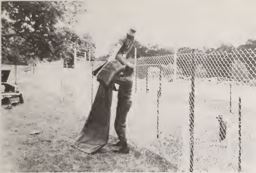
Figure 205. Climb to Throw Heavy Tarpaulin over Concertina Wire ; Test F6
