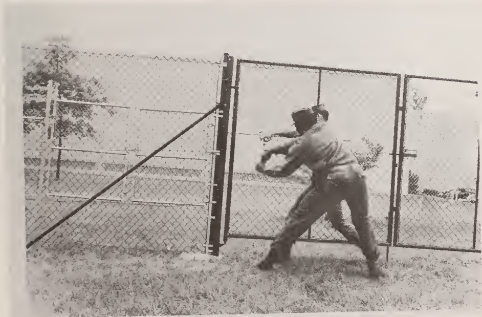
Figure 195. Pulling Metal Fabric Away from Frame; Test F4
