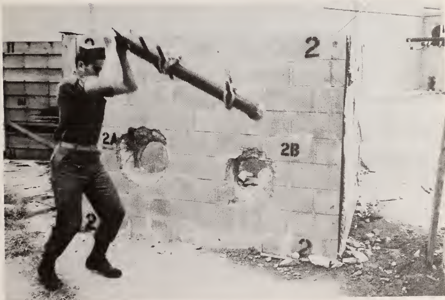
Figure 41. Test 5K. Single Man Using Suspended Battering Ram, Raising Center of Gravity 24"
