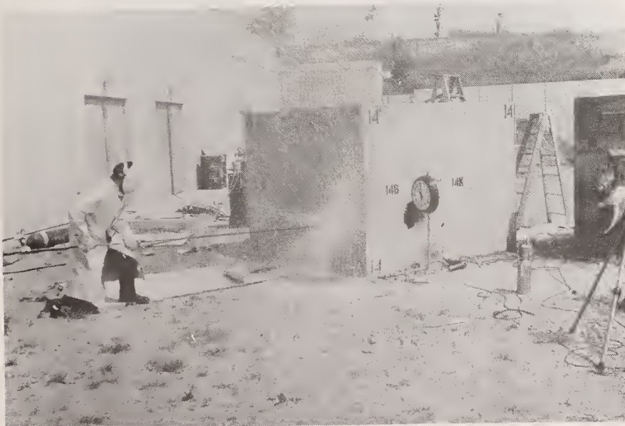
Figure 116. Test 13D. Beginning of Burning Bar Attack
