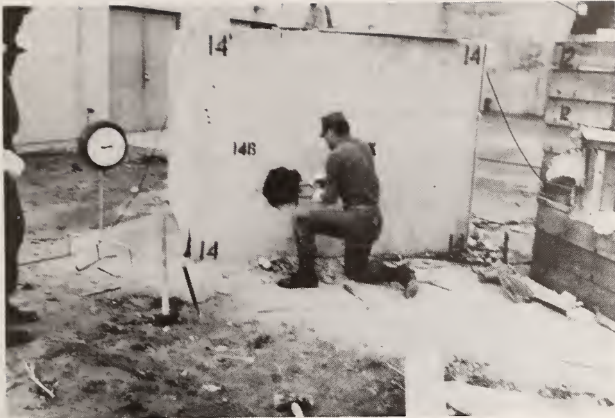
Figure 130. Cutting Reinforcing Rod with Bolt Cutters ; Test 14B
