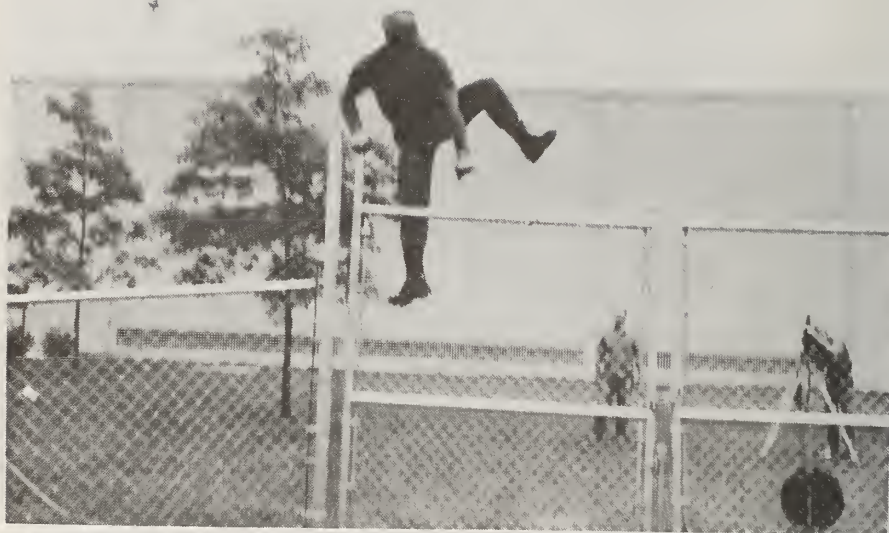
Figure 171. Gloved Hand Climb Over at Gate where Barbed Wire Outriggers Were Vertical; Test F1
