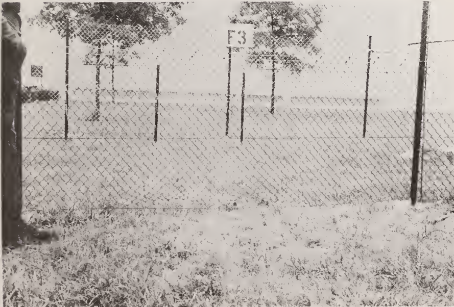
Figure 182. Appearance of Fabric after Dropping ; Test F3
