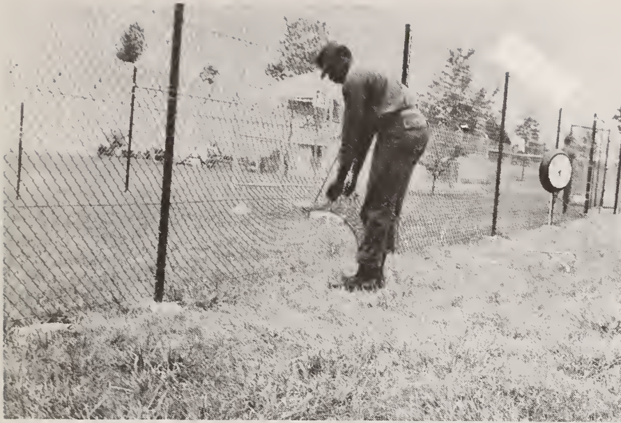
Figure 181. 25" High Opening Produced in Lighter Gauge Material; Test F3
