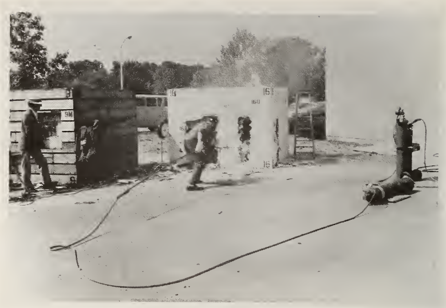
Figure 150. Burning Bar Cutting Through Steel Reinforcing; Test 16U
