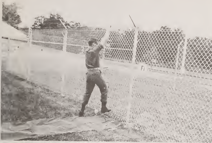
Figure 159. Climb Over Fence Using Wire Ladder; Test F1
