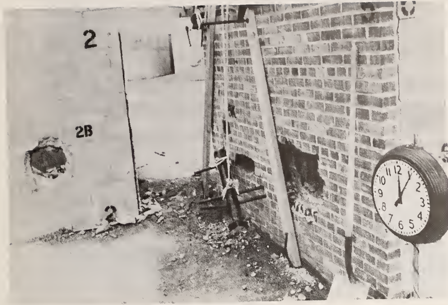
Figure 40. Test 5K. Battering Ram Suspended from A-Frame
