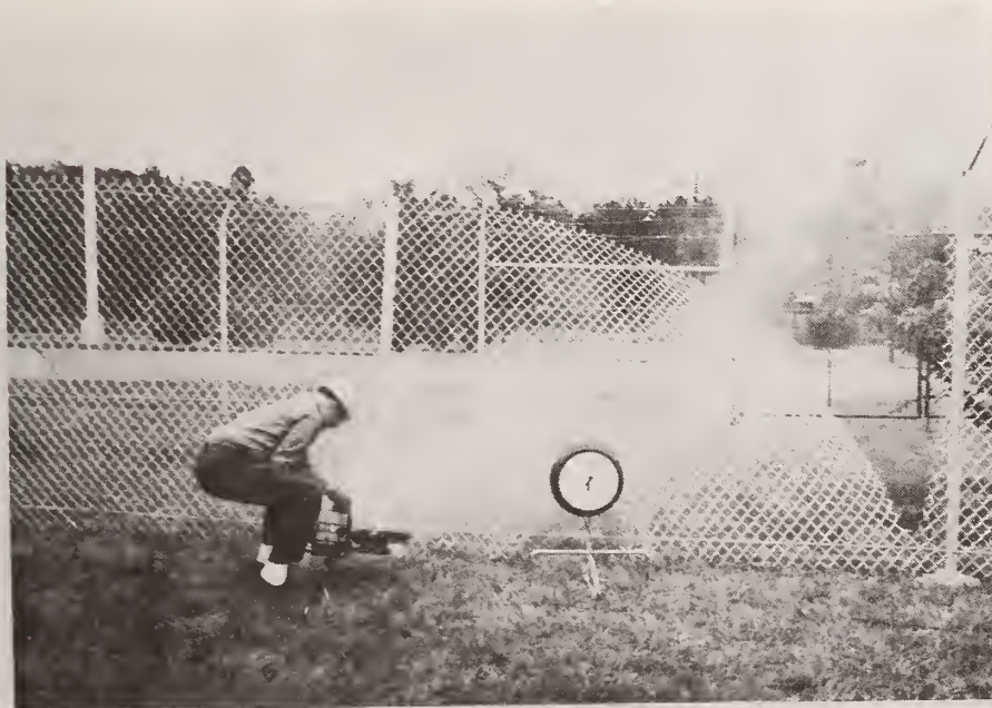
Figure 170. Abrasive Wheel Saw Used to Cut Nearly Full Height of Fabric and also to Cut Off One Intermediate Post; Test F1
