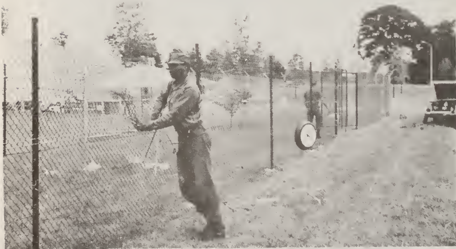
Figure 184. Pulling Down Fabric from Top Tension Wire in Preparation for Climb-over; Test F3
