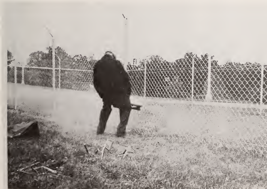
Figure 166. Abrasive Wheel Saw in Use; Test F1
