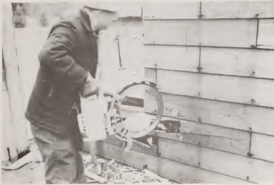
Figure 71. Panel 9. Hubless Saw Attack; Test 9M
