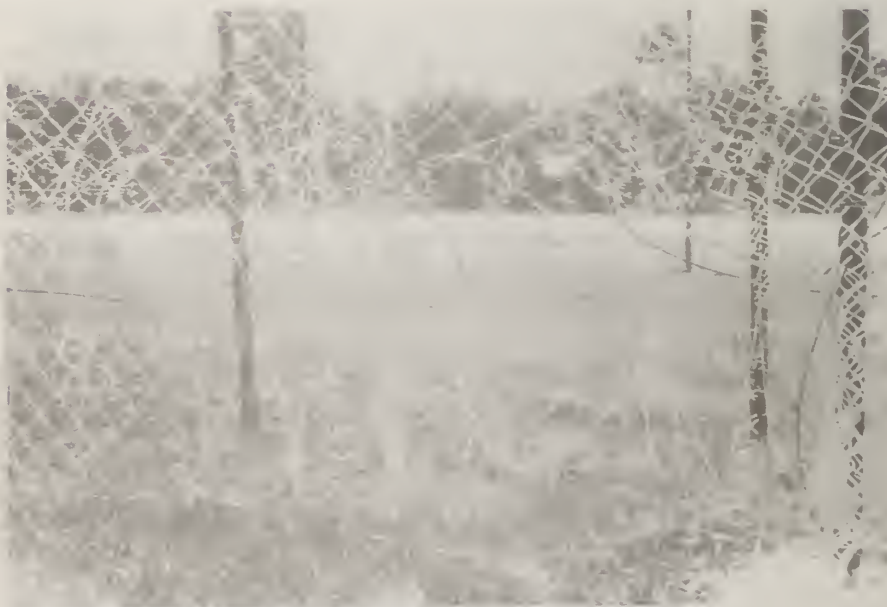
Figure 204. Concertina Wire Spread Apart, Hooked to Other Strands Resulting in Crawl Through Space; Test F6
