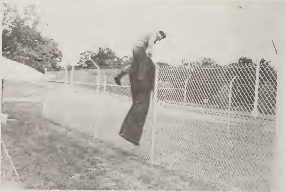
Figure 158. Climb Over Fence Using Tarpaulin as Protection against Barbed Wire; Test F1
