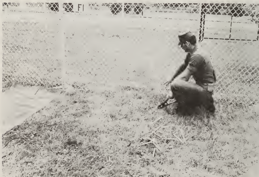
Figure 162. Opening Produced by Cutting 13 Wires with No. 14 Bolt Cutters; Test F1
