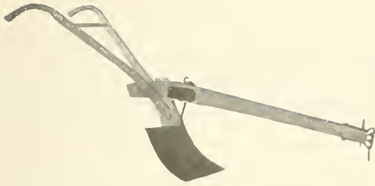
Figure 3.—RECONSTRUCTIONS OF JOHN DEERE'S 1837 PLOW. For a discussion of the position and attachment of the handles see p.24. (Deere & Company photo.)
