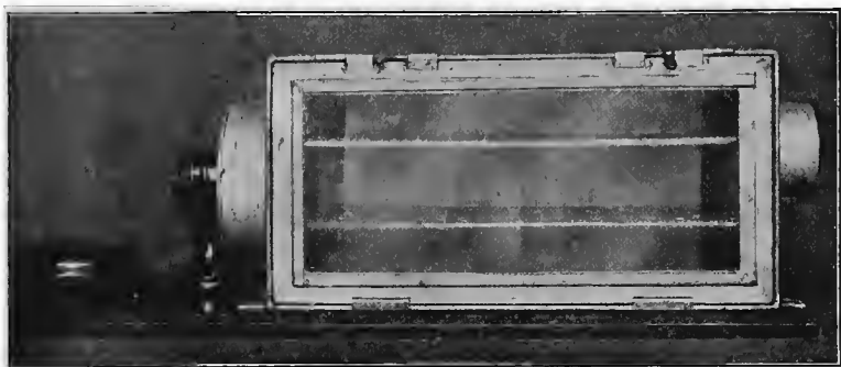
FIG. 2.—Drying chamber with fan for use in an incubation chamber.
