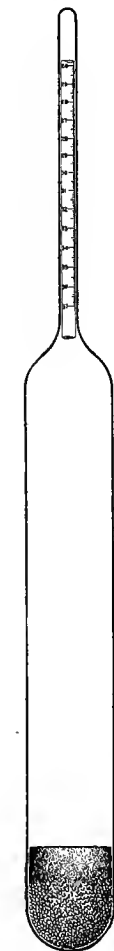
FIG. 4.—Shaw and Eckel's lactometer. Bull. Bur. An. Ind. , 134, U. S. Dept. Agric.
