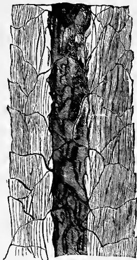
FIG. 60.—Sheep's wool (highly magnified), showing the cortical scales and the medullary tube.
