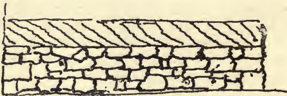
COB COURSE, OR SCAR, SHOWING DIAGONAL LAYERS.
