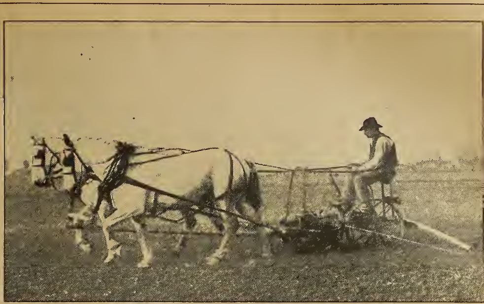
Nearly all planters have a variable drop by which the operator can change the drop so as to plant two, three, or four kernels in a hill without stopping the team
