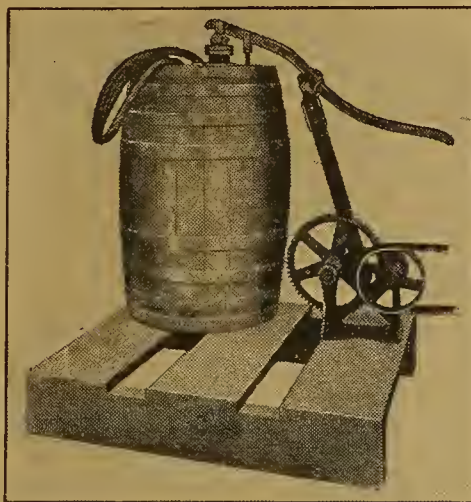
This simple jack enables the gas engine to pump spray mixture, saving one man
