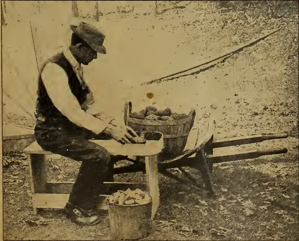
This home-made device for cutting seed potatoes consists of a bench with a knife inserted so that potatoes can be pushed against the edge of the blade
