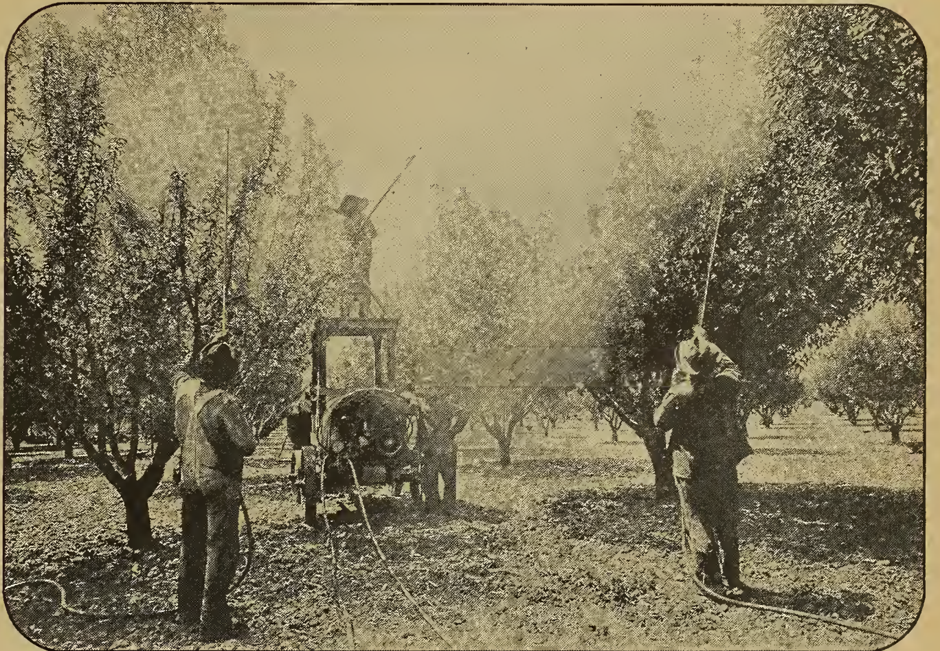
I N HANDLING large orchards the man without a power sprayer can't give the pests "knock-out drops" fast enough to put them out of business, and keep them out. This is a four-man power outfit, one man to drive and attend the machinery, and three men to spray. A crew of this size can handle 125 acres of orchard, and apply more than 100 wagon loads of spray mixture a week if necessary. A pressure of 200 to 300 pounds to the square inch can be maintained
