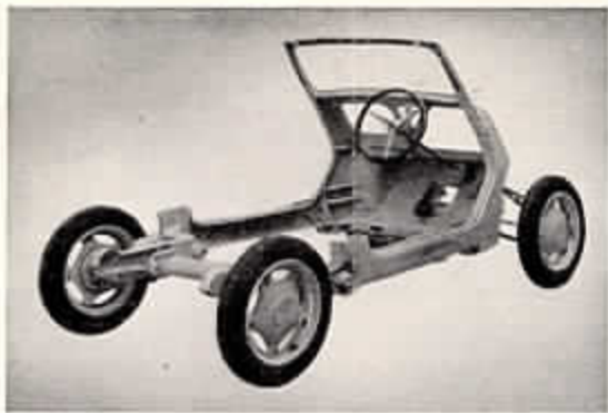
Featuring the Construction and Rigidity of the Chassis Frame.
