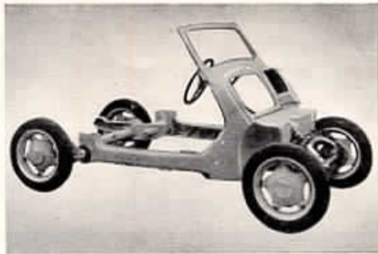
Featuring the Construction and Rigidity of the Chassis Frame.
