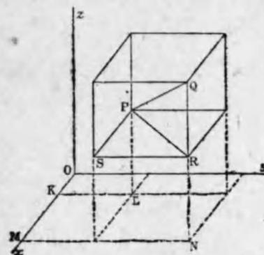
$$\begin{aligned} PQ^2 &= PR^2 + RQ^2 \\ &= PS^2 + SR^2 + RQ^2 \\ &= (OM - OK)^2 + (MN - KL)^2 \\ &\quad + (NQ - LP)^2 \\ &= (x_2 - x_1)^2 + (y_2 - y_1)^2 + (z_2 - z_1)^2 \end{aligned}$$
