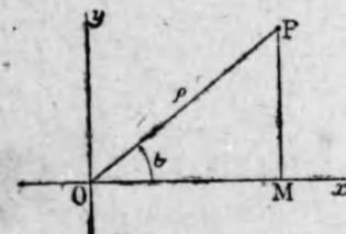
$$\left. \begin{aligned} x &= \rho \cos \theta \\ y &= \rho \sin \theta \end{aligned} \right\} \dots(4)$$
