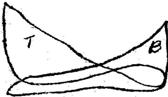
H.P. Card showing effect of broken bottom bar.
