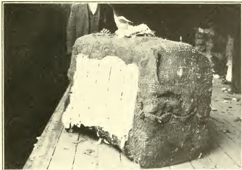
FIG. 1.—BALE AS RECEIVED AT THE COMPRESS FROM THE GINNERY AFTER BEING CUT AND SAMPLED.
