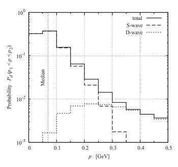
FIG. 17. Momentum distribution of the deuteron with the AV18 wave function [56]. The histogram shows the probabilities to find a nucleon with momentum  $p_1 , Eq. (A12), for <math>p_{1,2}$  in steps of 50 MeV. The constant values shown at  $p_1 give the value of <math>P_d(p_1 for that range. The median momentum is indicated by a vertical line.$
