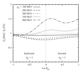
FIG. 14. The ratio of the distorted spectral function to the IA spectral function,  $S_d[\text{dist}]/S_d[\text{IA}]$ , Eqs. (6.52)–(6.55), as a function of the cosine of the recoil momentum angle in the deuteron rest frame,  $\cos\theta_{pq}$ , for several values of the recoil momentum modulus  $p_p \equiv |\boldsymbol{p}_p|$ . The distorted spectral function includes the IA, FSI, and FSI<sup>2</sup> terms
