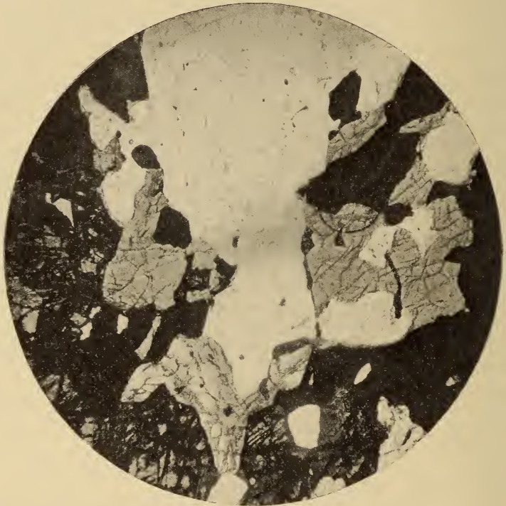
FIG. 1. Microphotograph of thin-section, showing plagioclase (white) almost entirely surrounded by sapphirine (gray) either as a narrow band or as larger grains between it and the ilmenite (black) or rutile (dark, mottled). The plagioclase shows many minute microlites of spinel. Magnif. about 90; ordinary light.
