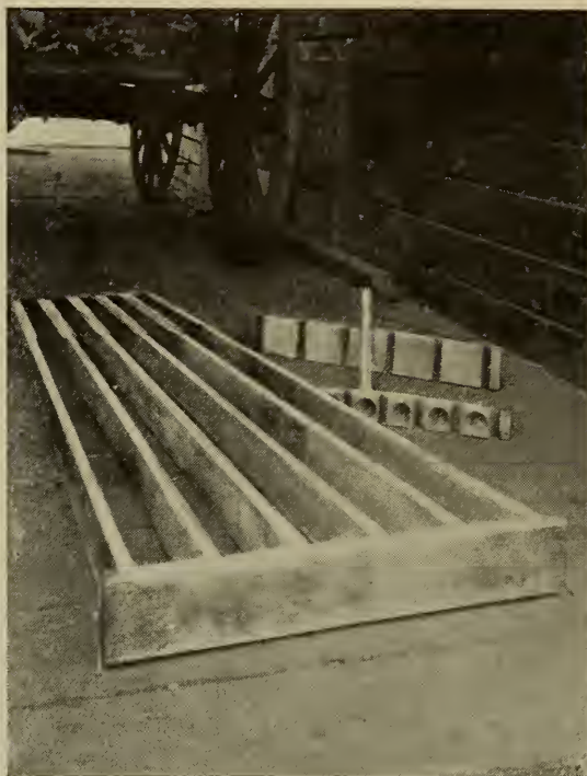
31. A home-made mold which will give the owner durable posts.
