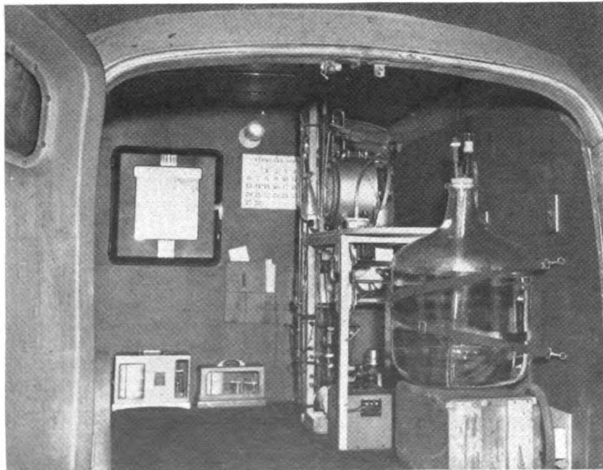
The use of a mobile laboratory, lent the PHS by the Utah State Health Department, facilitated the engineers' research. The picture shows a Thomas Recorder.
