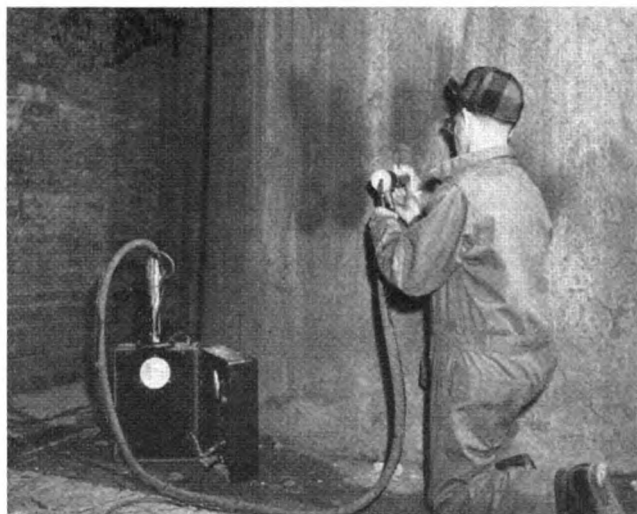
An engineer takes an electrostatic precipitator sample in a stack of the steel mill.
