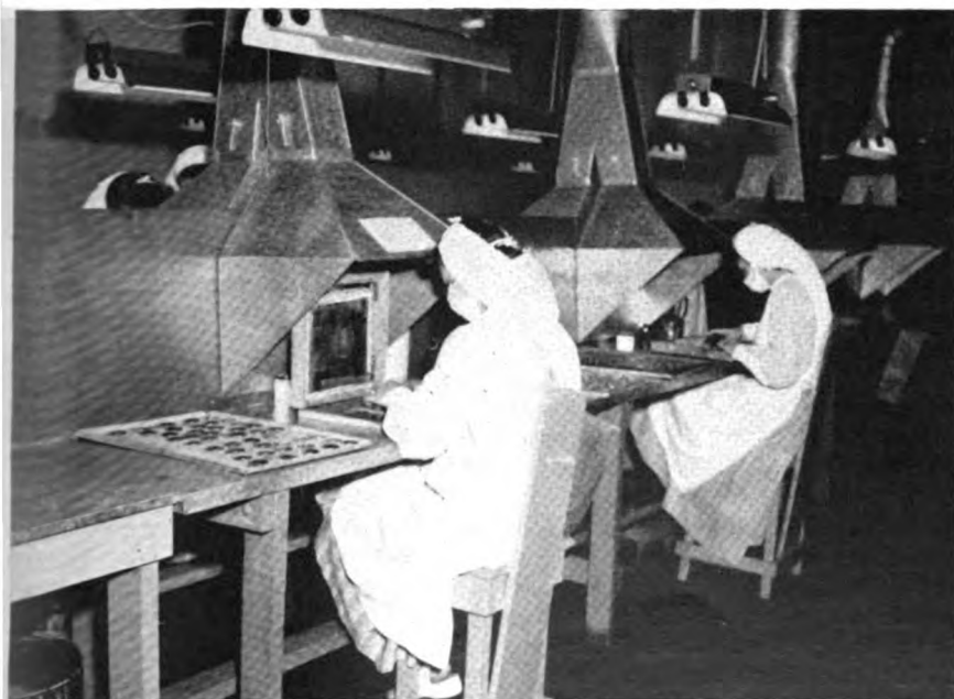
Radium dial painters at work, well protected by protective clothing and local exhaust ventilation.
