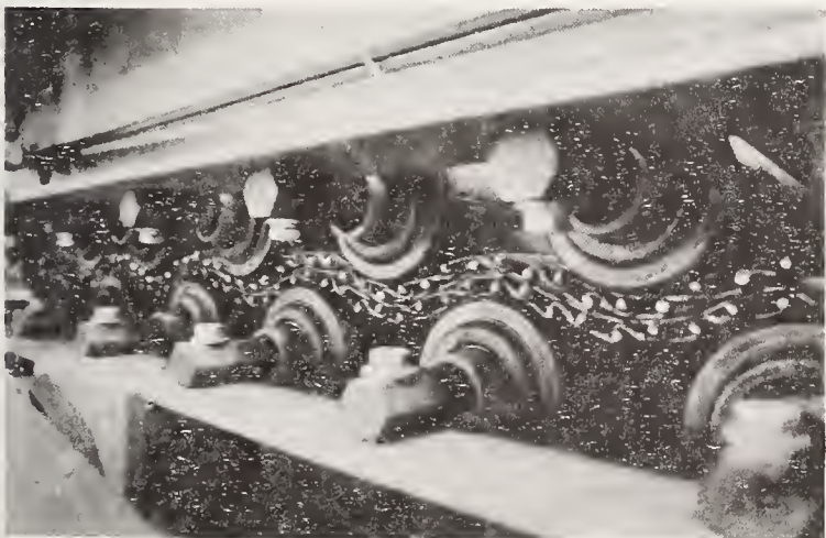
Fig. 21 - Side view of double mesh belt unit showing "working" action taking place on both sides of SMC sheet
