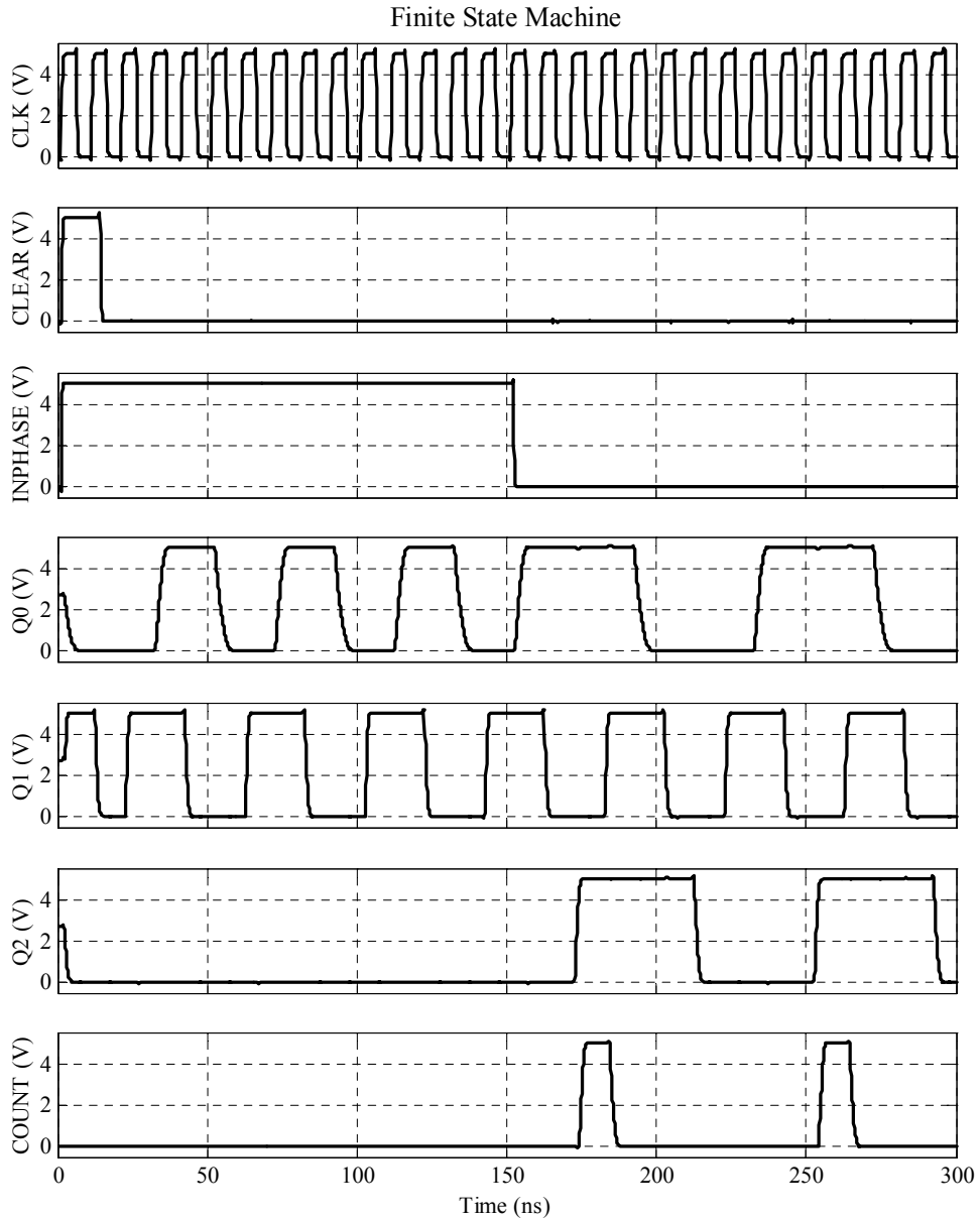
Figure 2.40 Finite state machine simulation.
