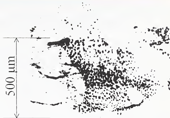
Figure 1: USAXS image of creep cavities in copper.
