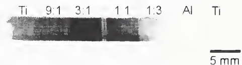
Fig 1. GaN strip with array of Ti:Al metallization pads
