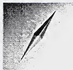
Magnified view of Knoop indentation in a new gold micro-hardness test block developed for the electronics industry.
