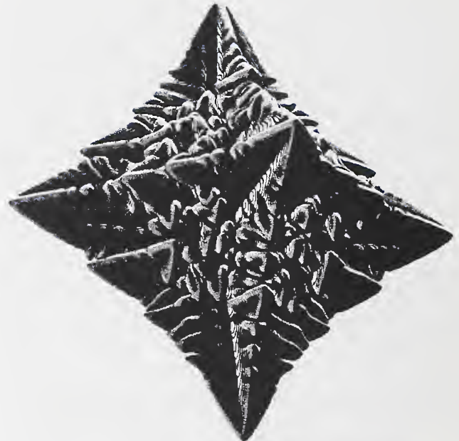
Figure 2: 3D phase field calculation of a binary alloy dendrite
