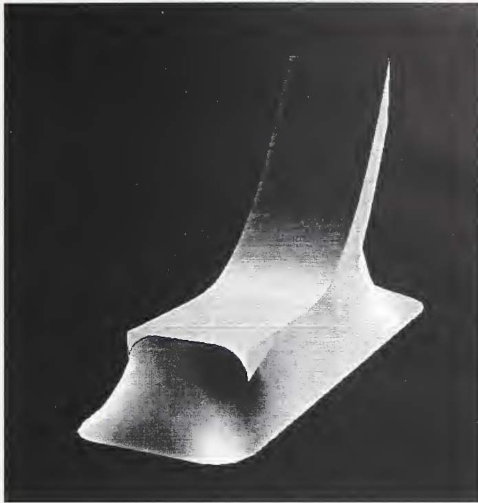
Surface Evolver calculation of the geometry of solder wetting a gull-wing lead. The shape of the liquid surface depends on the surface energy and the contact angle with the substrate.
