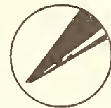
Ordinary needle after playing one record. Point worn blunt. Will injure record.
