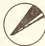
Ordinary needle after playing one record. Point worn blunt. Will injure record.
