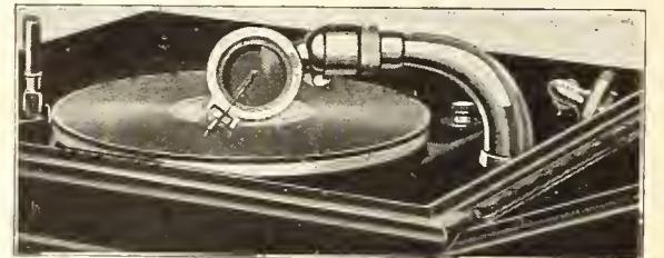
Showing Reproducer of Jewell Needle Equipment in Position for Playing Lateral Cut Records on Edison Phonograph
