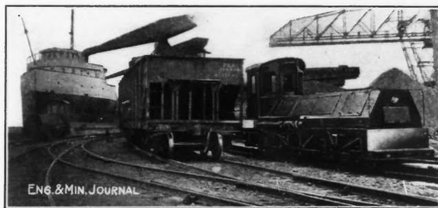
ELECTRIC LOCOMOTIVE PUSHING AN ORE CAR ON A PARALLEL TRACK
