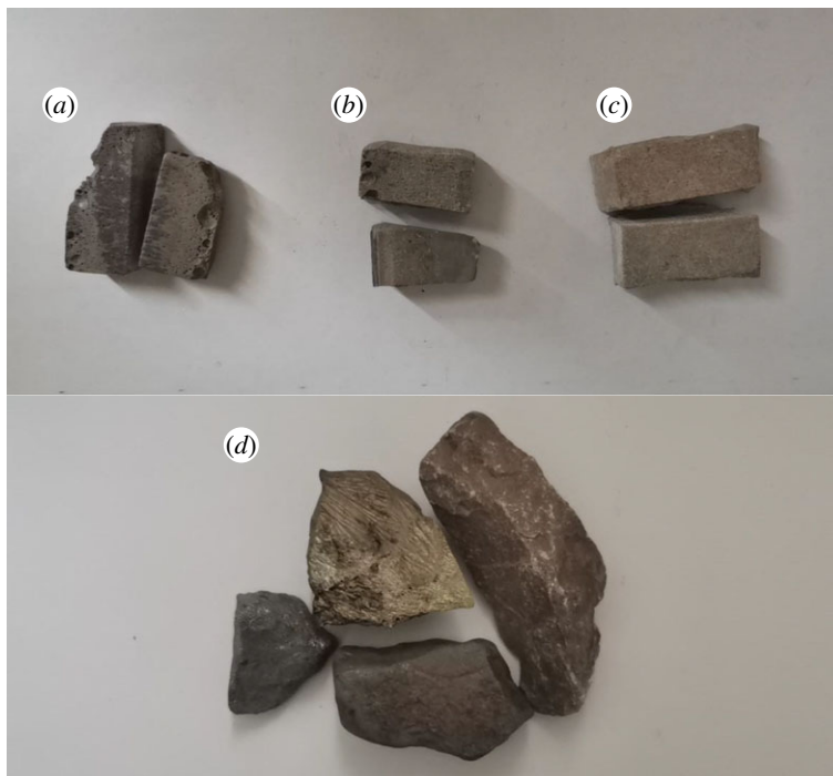
Figure 1. Fluorine-containing slag. (a) Remelting electroslag, E1; (b) remelting electroslag, E2, E3; (c) remelting electroslag, E4; (d) continuous casting mould flux.
