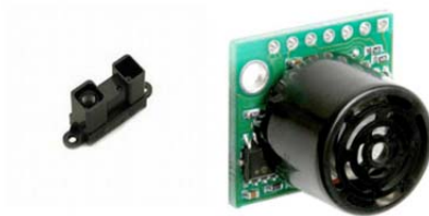
Figure 29. SHARP GP2D12 IR Sensor (Left) - LV-MaxSonar-EZ0 Sonar Range Finder (Right). After [54].
