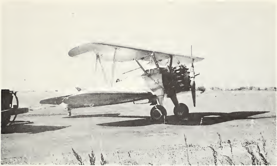
Figure 1. --The agricultural biplane used for the water-drop tests.
