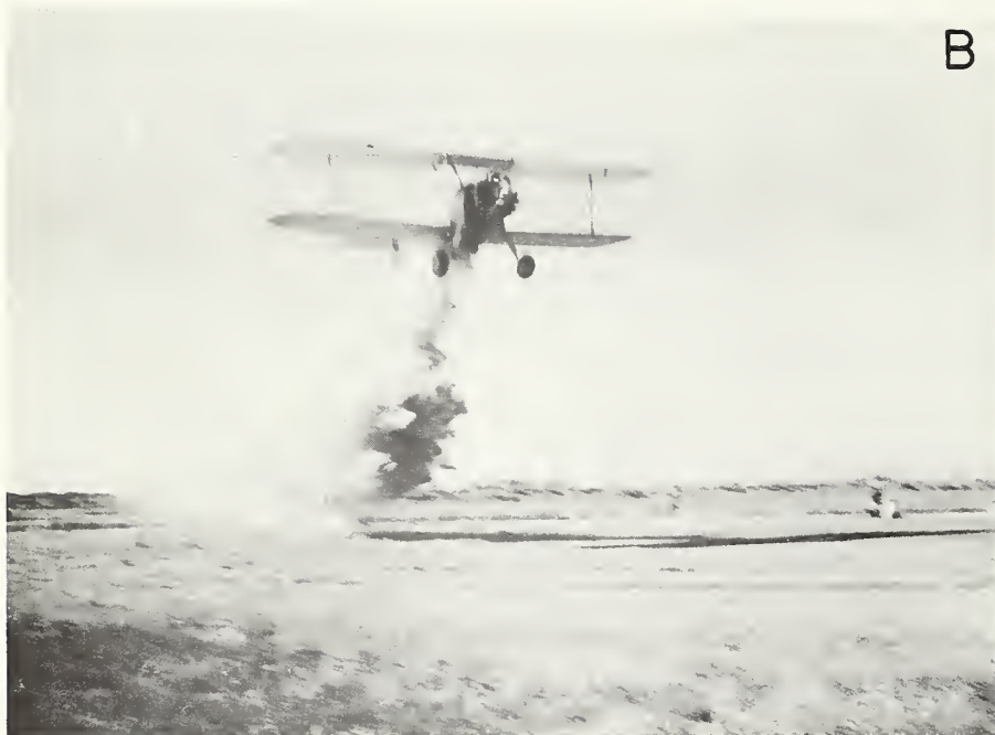
Figure 4. --Dropping water and retardant; note difference in break-up of the liquid A , water; B , retardant.
