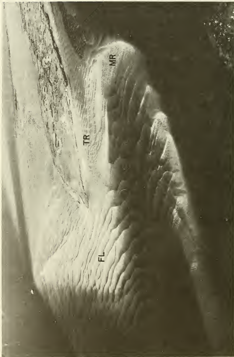
Figure 13. Aerial View of a Part of Middle Ground Flood-Tidal Delta. Location of three diving stations are shown. Bed form morphology is: FL - flood-oriented sand waves, TR - transition bed forms, and MR - megaripples.
