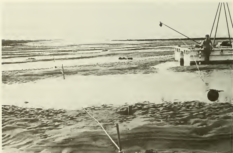
Figure 6. Pipe and Rope System in Place at an Intertidal Diving Station
