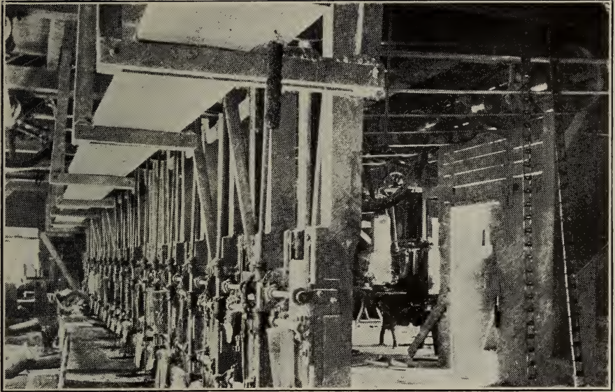
Fig. 30 —Interior of excelsior factory, showing billets in place in excelsior machines.
