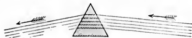
FIG. 20. — Showing how rays of light are refracted in passing through a prism.
