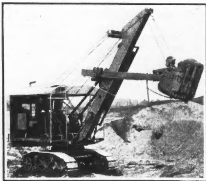
Convertibility from shovel to crane is a feature of this excavator, which is tractor-mounted and gasoline-engine driven
