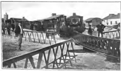
A Steam Train of Mono-rail Type now in Operation at Ballinacorney in Ireland The railway, which is about three miles long is situated by steam with rail the last century track between Manchester and Liverpool will be by steam. The engine and carriages are along in passenger tracks across the steel rail which is raised above other feet from the ground. The steel rail is used
