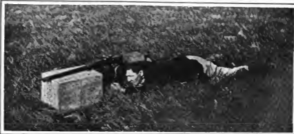
Shooting over a Row by means of the Hyposcope—The Marksman is invisible to the Target
