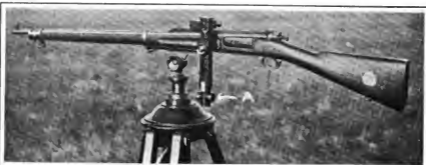
The Hyposcope attached to the Rifle. A is the Sight through which the Marksman gets his Bearings
