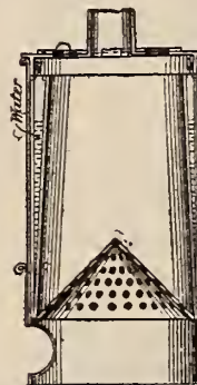
Water Tank Fumigator.
