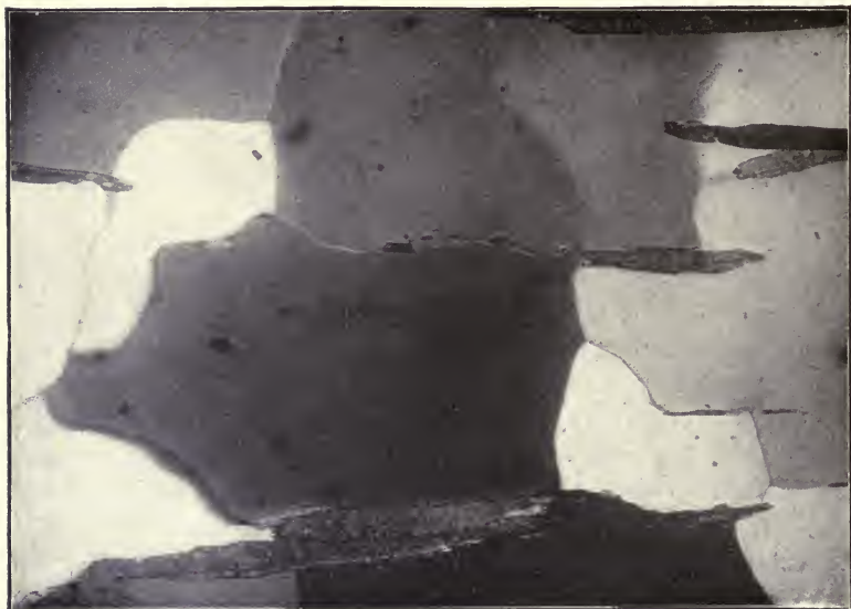
FIG. 38. Photomicrograph of micaceous and quartzose schist showing recrystallized quartz. From Hoosac, Mass. The view illustrates in detail the relation of recrystallized quartz grains to recrystallized mica flakes. The mica flakes for the most part separate different quartz individuals, but they may be seen to bound two or more individuals and to project well into them. It is not probable that such a relation could be brought about by granulation, slicing, or gliding, and it seems best explained by recrystallization.
