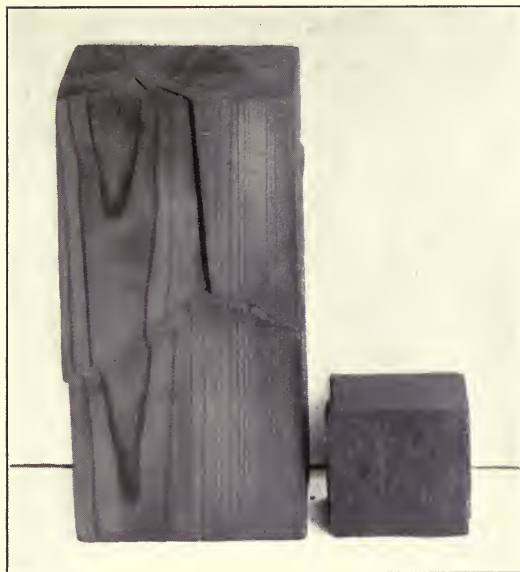
FIG. 3. Results of crushing wooden blocks by non-rotational strain. Note tendency of fractures to follow shearing planes 45^\circ to the pressure (which was from above) regardless of the grain of the wood.
