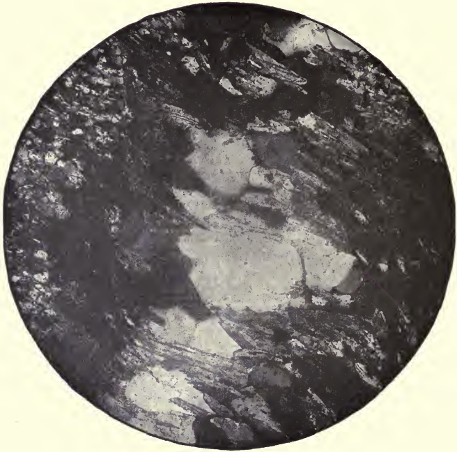
FIG. 45. Photomicrograph of micaceous and quartzose schist with cleavage developed across original bedding, from Little Falls, Minn. A graywacke-slate, in which the banding has been marked by difference in texture as well as in composition, has been subjected to deformation, with the result that a cleavage has been superposed at right angles to the original bedding. Originally the longer diameters of the particles of the bedded rock were parallel to the bedding. Accompanying the development of flow cleavage most of the constituents of the rock have been recrystallized. The quartz particles shown in the light band have been drawn out with their longer diameters nearly at right angles to the former plane of their longer diameters, and abundant new mica has developed with its greater diameters and mineral cleavage normal to the plane of bedding.
