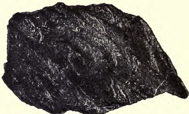
FIG. 28. Fault-slip cleavage in gneiss from southern Appalachians. The gneiss has been closely crenulated and the minute folds may be observed to pass into minute faults which now represent planes of fracture cleavage. The faults may have been cemented or may have been welded by actual pressure. Parallel to the faults there has also been developed a parallel arrangement of the mineral particles, perhaps due in part to the slipping along the fault planes, and it is exceedingly difficult to distinguish between the fracture cleavage and the flow cleavage.
