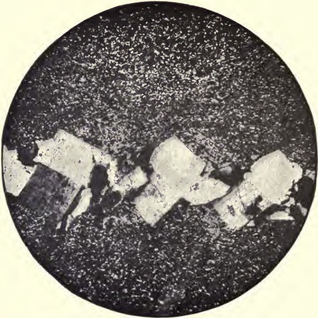
FIG. 40. Photomicrograph of schistose quartz-porphry showing sliced feldspar phenocryst in planes inclined to the prevailing cleavage. After Futterer. (Fig. 2, Pl. III of Ganggranite von Grosssachsen und die Quarzporphyre von Thal in Thüringer Wald : Mitt. Grossh. Badischen geol. Landesanstalt, Vol. 2, Heidelberg, 1890.)
