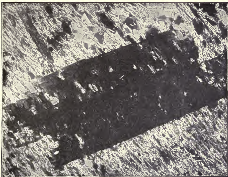
FIG. 44. Photomicrograph of chloritoid crystal in micaceous and quartzose schist from Black Hills. The chloritoid crystal here shown has developed later than the rock flowage producing the prevailing cleavage of the rock. The chloritoid has grown at the expense of the other constituents of the rock, using all the material necessary for its growth and leaving the excess of material in the form of inclusions, which retain their dimensional parallelism with the prevailing rock cleavage.
