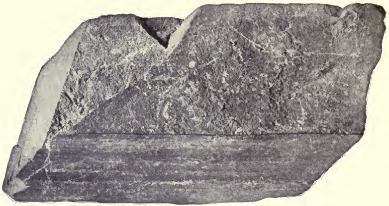
FIG. 34. Fracture cleavage developing polygonal blocks in slate previously possessing flow cleavage.
