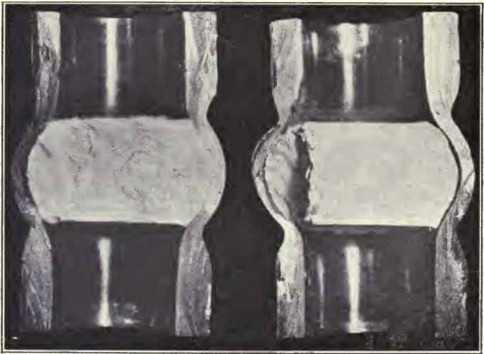
FIG. 1. Flowage of marble. After Adams. a. Columns of marble before and after deformation. b. Deformed column of marble as it appears in the steel jacket.
