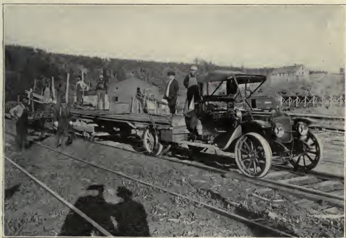
THE ADAPTABLE MOTOR-TRACTOR Equipped with flange wheels and hitched to a flat-car train on a logging railroad, it makes a bully motor-truck of real hauling capacity.
