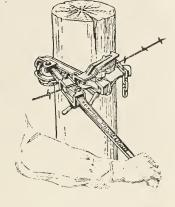
not matter how much slack there is in the wire, operator can finish the job without resetting machine, as the Whitesel has a continuous pull. resetting
