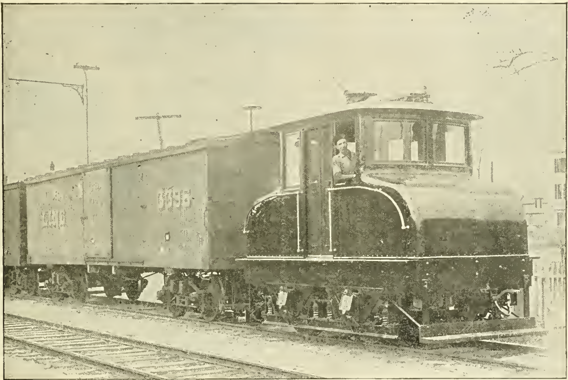
THIRTY-TON ELECTRIC LOCOMOTIVE. BUILT BY THE GENERAL ELECTRIC COMPANY.
