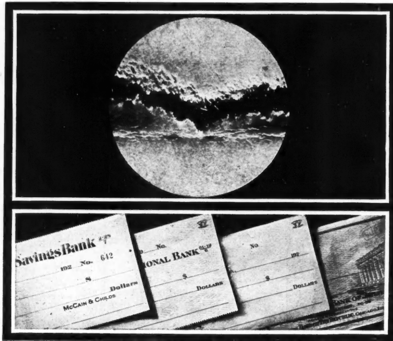
The long fiber and small amount of sizing in this superlatively strong new paper are illustrated by this micro-photograph
