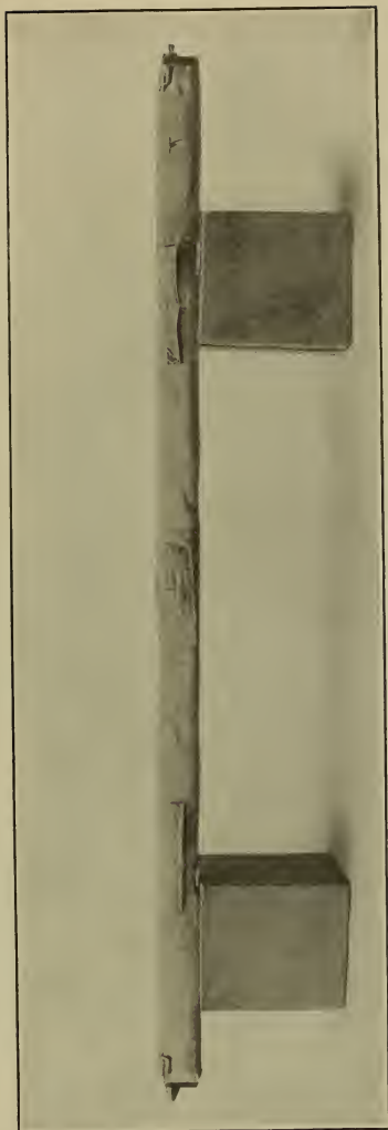
FIG. 35.—SCHOTT FIVE-METER COMPENSATION BASE BAR
