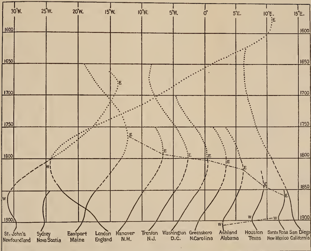
FIG. 1.—TYPICAL CURVES SHOWING THE SECULAR VARIATION OF THE MAGNETIC DECLINATION IN ENGLAND AND NORTH AMERICA FROM THE DATES OF THE EARLIEST OBSERVATIONS
